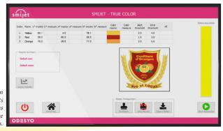
Smijet control screen automatically points out color areas exceeding tolerance thresholds.
